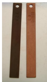
Fig. 1 – Circuit carbon steel and copper corrosion coupons.
