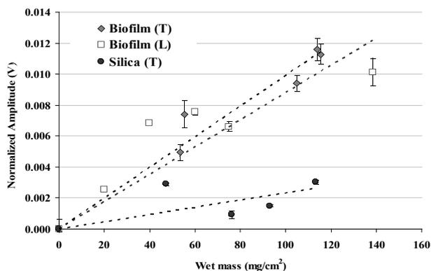
Figure 2: Variation of the MSS normalized amplitude with the wet mass per unit of area: *Pseudomonas fluorescens* biofilm under turbulent flow ( $\blacklozenge$ ), *Pseudomonas fluorescens* biofilm under laminar flow ( $\square$ ) and silica deposit under turbulent flow ( $\bullet$ )
