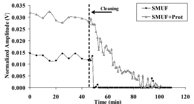
Figure 3: Cleaning of SMUF and SMUF with whey protein deposition curves assessed with the MSS
