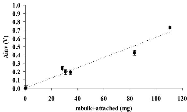
Figure 4: Relation between the  $A_{inv}$  and the mass of shampoo that remains in the flow cell after the cleaning procedure ( $R^2=0.9633$ )
