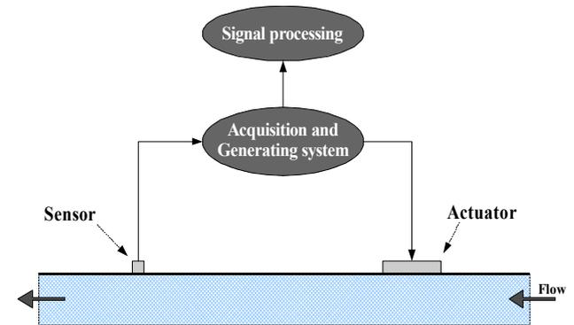
Figure 1: schematic representation of the MSS elements (actuator and sensor) and of the generating/acquisition system
